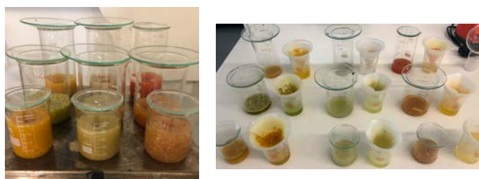
Figure 1. Maceration of pumpkin residues using ethanol/water 80:20 as extraction solvent.
